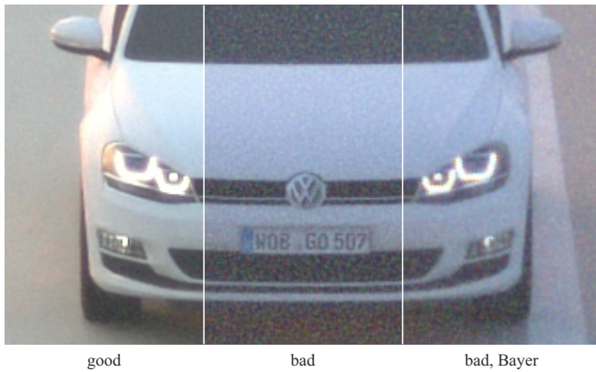
(c) Three of the four qualities (good, Bayer not shown) computed per geometric path tracing result. The “good” quality set has optimal balance and low noise levels. Bad introduces AEC and white balance deviations, lens flares and higher noise levels. Bayer introduces demosaicing effects from a BGGR Bayer pattern (visible, e.g., in the headlight fringes).
